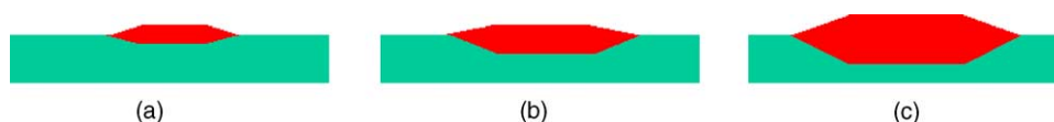
Fig. 5. Schematics of the oxide islands formed at the different oxidation temperatures: (a) 450 °C; (b) 550 °C; (c) 650 °C.
